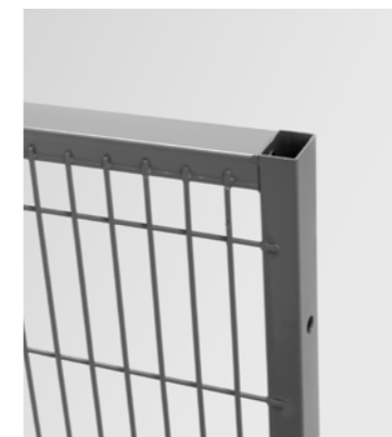
ST30 MESH PANEL The ST30 mesh panel has a classic look with the mesh size of 20×100 mm fixed to a 30×20 mm frame. Available in two standard heights, 1,250 and 2,050 mm in up to 8 widths.
