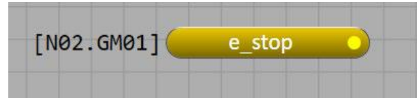
Illustration 13.31: A reference with N02.GM01 as source memory. Note the color and tag match the source memory.
