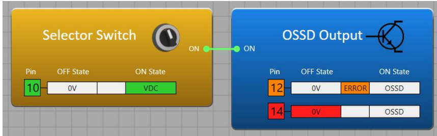
Illustration 13.54: OSSD Output in ERROR state due to an external error on terminal 12 (short circuit to 24V).
