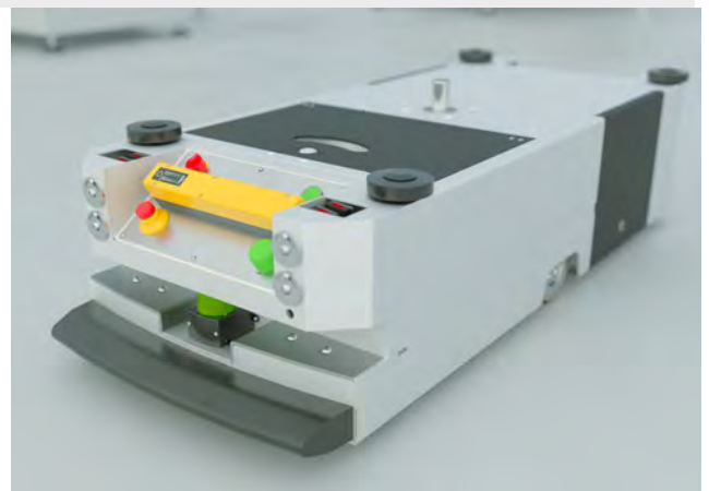
Safety Simplifier for safe control and monitoring on self-propelled floor conveyor vehicles.
