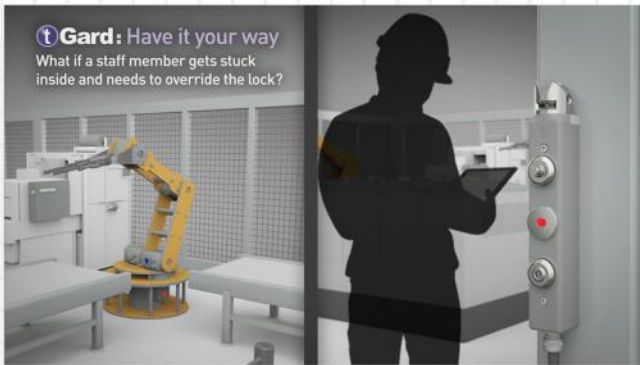
Guard door is open and operator enters cell.
