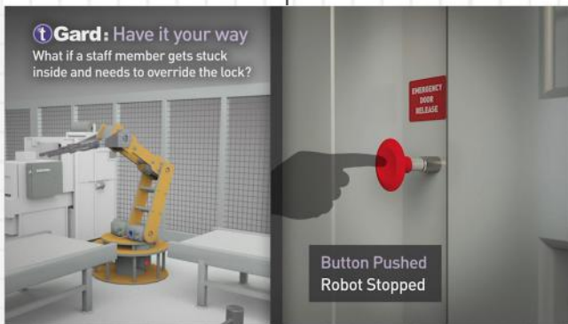
Operator hits escape release button, overriding solenoid and stopping machine.
