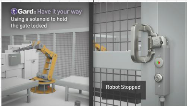
When machine is at end of cycle, solenoid is energised, breaking safety contacts and machine stops.
