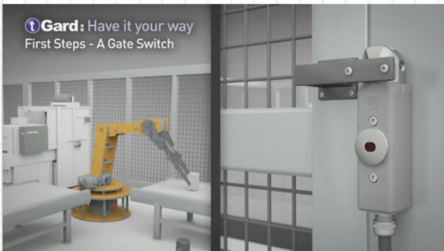
Guard door closed, contacts made and machine runs.
