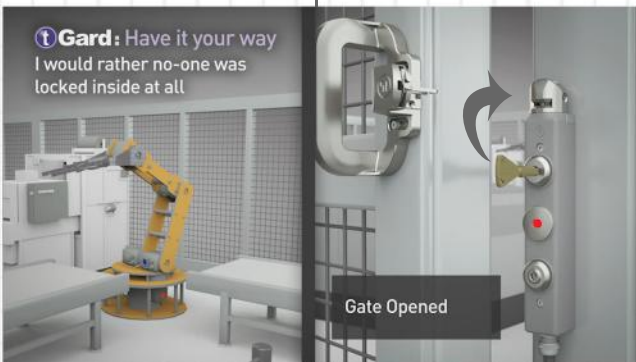
Solenoid is energised, safety circuits interrupted to stop robot. Key can then be released and door opened.
