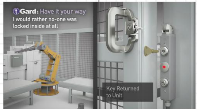
Only when operator exits the guarded area and returns key to the interlock, can the door be closed and locked.
