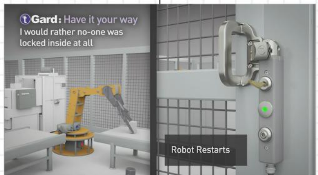
With key back in place, door is closed and locked and robot restarted.
